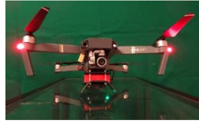
DJI Mavic Pro with embedded Parrot Sequoia camera (multispectral)
