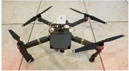
DJI Mavic Pro with sensing pollution, NIR spectrometer, etc
