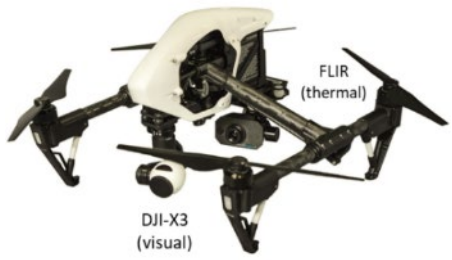
DJI Inspire 1/2 + FLIR (thermal imaging) and pollution/climate sensing
